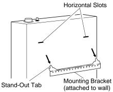
Figure 16 - Mounting Heater Onto Mounting Bracket
